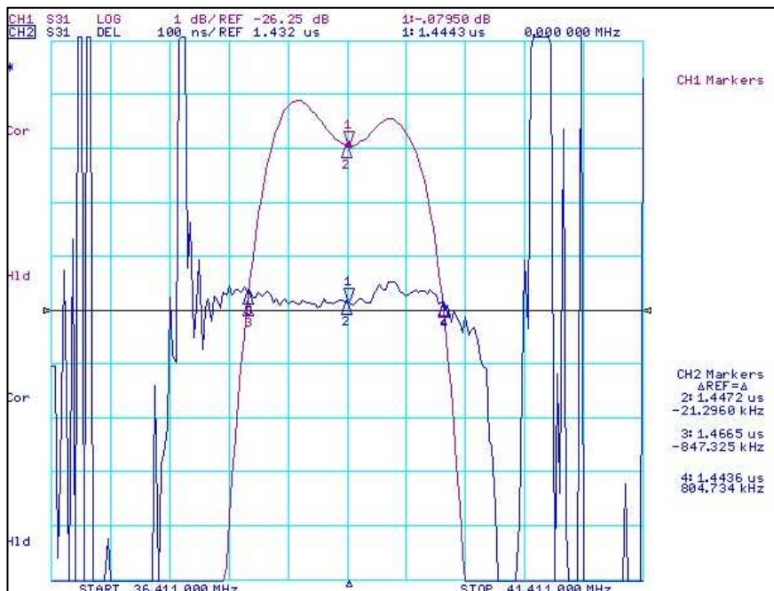
Fig 2. S21 Response Horizontal: 0.5MHz/Div Vertical: 1dB/Div 100ns/Div
