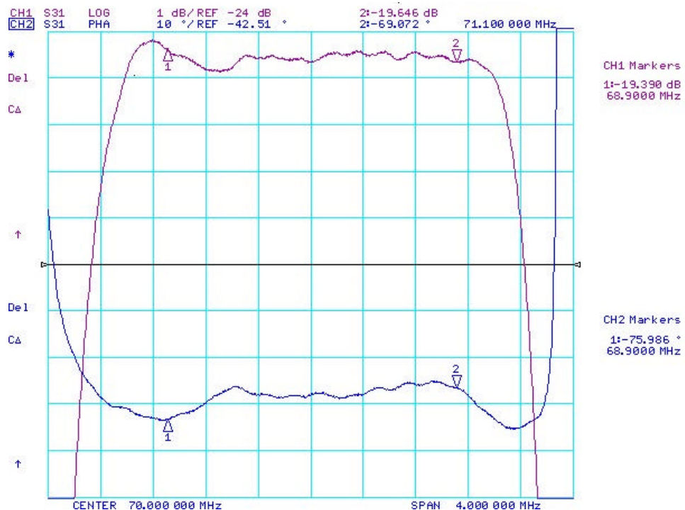
Fig-2 Phase linearity and Ripple, Horizontal:0.4MHz/Div. Vertical: 1 dB/Div Vertical: 10deg/Div
